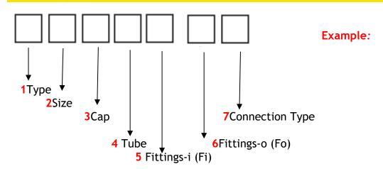
SENH Type Column, fittings are 1/4" and quick connection type, stainless steel tube, has stainless steel caps and the sizes are A.
